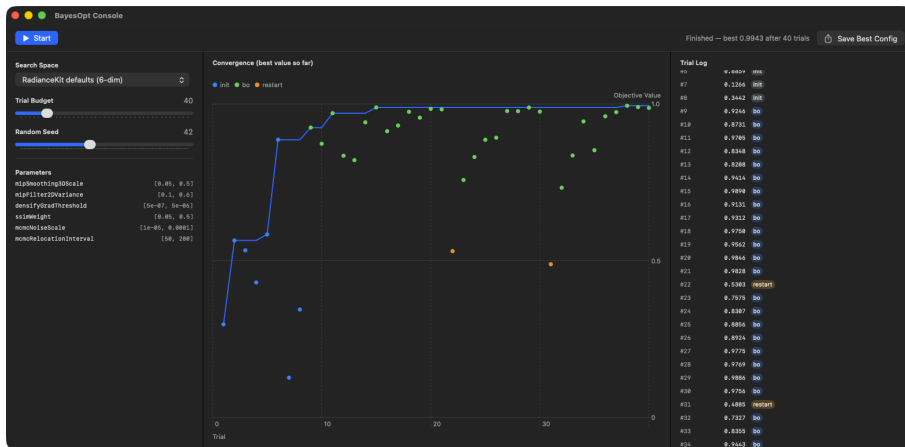
图 25 BayesOpt 控制台经过 40 次试验 — Convergence 图陡升到 Trial 15, Best Value 0.9943, Trial Log 含 init/bo/restart 标签
